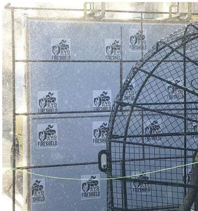
Figure 3 – AAMA 501.1, Dynamic Water Penetration Test
